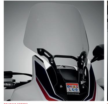
**TOURING SCREEN** Taller touring screen improves wind protection and reduces buffeting. Offers an 85 mm increase in height and a 30 mm increase in width compared to the standard screen.
