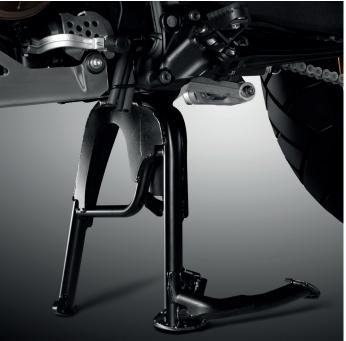
MAIN STAND A Main Stand allows secure parking on a variety of ground surfaces and assists with maintenance.
