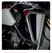
LOWER DEFLECTOR Polyurethane deflector designed to deflect hot air from the radiator away from the rider in order to improve comfort.
